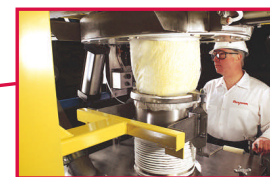
Prevent dead spots and promote flow with TELE-TUBE® telescoping tube*
