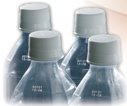
PET resin with little burning at a 9.3µm wavelength
