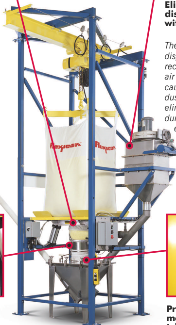
Cinch spouts concentrically with POWER-CINCHER® flow control valve*
