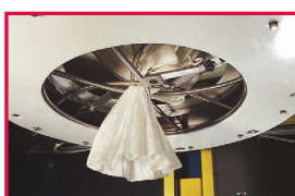
Cinch spouts concentrically with POWER-CINCHER® flow control valve*
